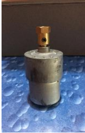
Fig. 12. Gear motor for the horizontal movement of the DAST.
