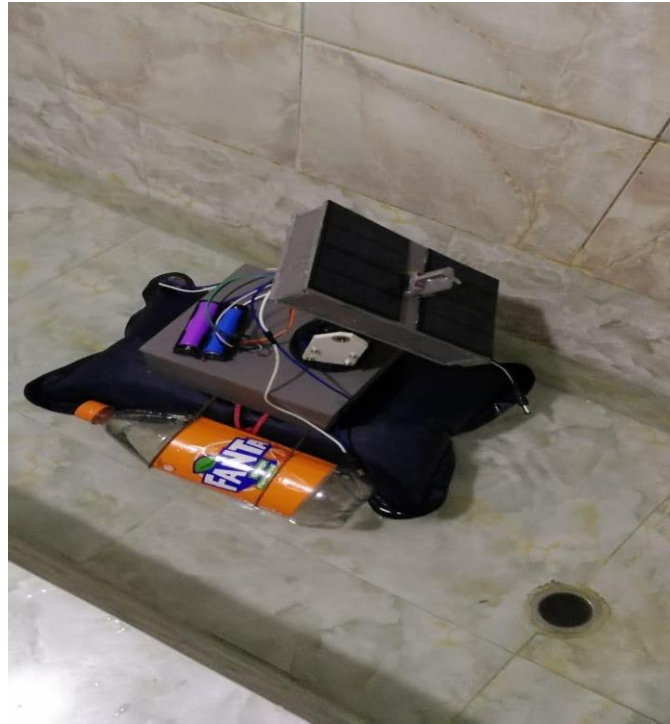
Fig. 15. Floating structure of the PV DAST system. The floating base was created using plastic bottles and floating pillow as a prototype.
