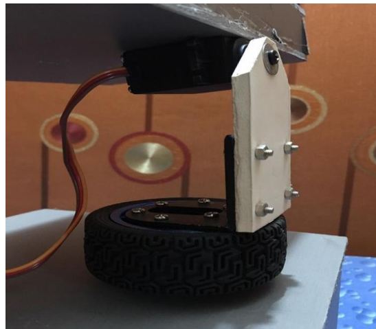
Fig. 11. Rotating base consisting of mechanical tire and servo motor
